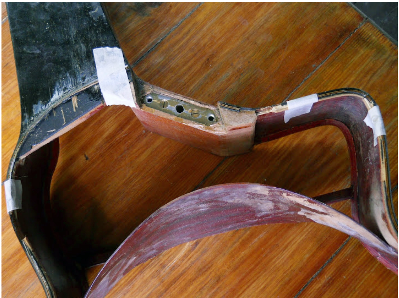
Above: It's also difficult to tell here how the neck is adjusted through the three holes in the back (seen earlier). The seating area of the neck was not photographed. But here you can see the thin, purple-stained reflector baffle glued to the sides.
