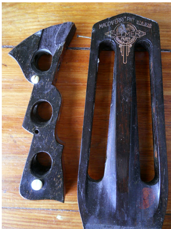
Like #275, the tip of the bass headstock was broken off; at right is Milani’s restored piece.
